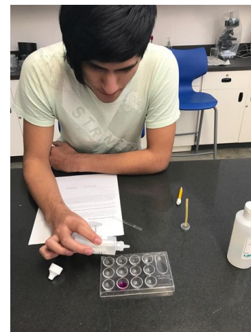
Jose learns about the chemical phenylthalein, which turns pink in bases, but remains clear in acids.
